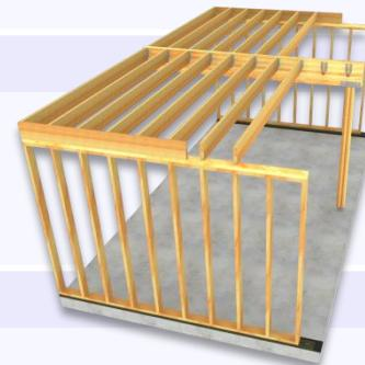
**L' OSSATURE D'UNE MOB DE TYPE PLATEFORME**
